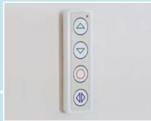
wireless landing controls
